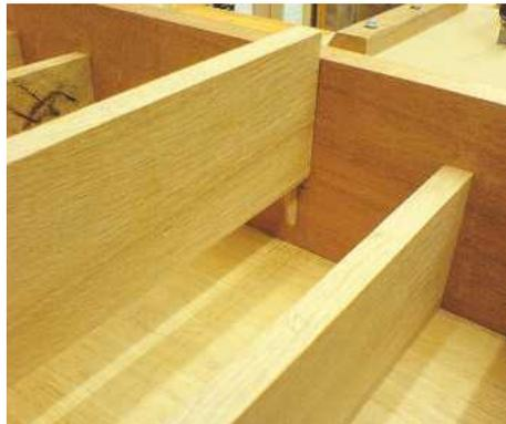
▲ Pic.15 Cut long slots using the biscuit joiner for the dividers and shelves to be slotted into
